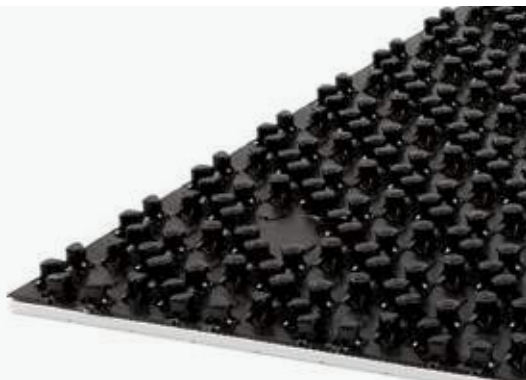
The Variotherm nap panels are pipe brackets, separating layers and thermal insulation (VarioNap) all in one. They are simply connected using a snap fastening system. They are also available without thermal insulation as VarioFix.
