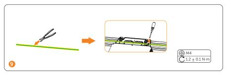
Step 8: Connect Multiple PV Modules to Microinverter
