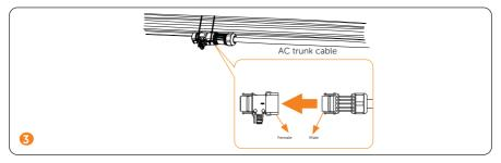
C) Band the AC trunk cable with cable ties. In order to better fix the AC cable, it is recommended to use more cable ties to band the AC cable.
