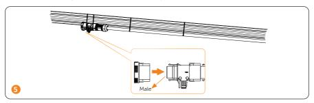
Step 5: AC Trunk Cable Connection
