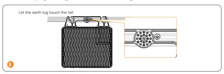
Method 2: Strip the PE cable, place the PE cable on the rail and fix it with screws.
