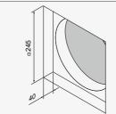
Create an opening for the flush-mounted housing on the interior wall, centred on the core drill hole, for installing the inner cover. Dimensions: 245 x 245 x 40 (W x H x D, mm)
