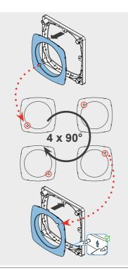
Remove the Flair Zero insert by unhooking it on all 4 sides.
