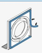
TIP: Do not apply the sealing tape until immediately before installing the base plate. This prevents the sealing tape from swelling too much and makes installation easier.
