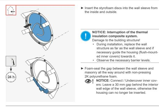
Depending on the **inner cover** to be used, cut off the excess, hardened mounting foam and protruding mounting wedges as follows:
