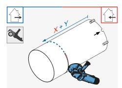
Cut the wall sleeve to the determined dimension X + a protrusion of Y on the exterior wall.
