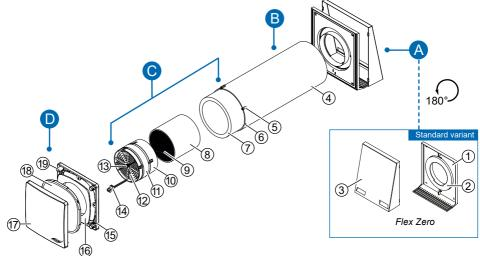
Figure 1: Overview of the iV14-Zero standard variant ventilation device
