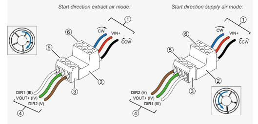
• The clamping screws of the plug connection are directed to the same side.
