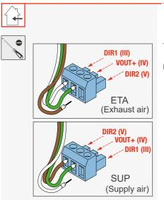
In paired operation, one reversible fan starts in extract air mode, the other in supply air mode. This start direction is determined by the different connection sequence of the three fan BUS cables in the plug-in connector.
