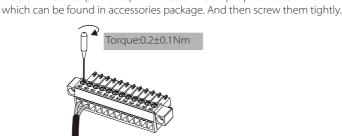
Step3. Trip the insulation from the communication wires, then insert one
