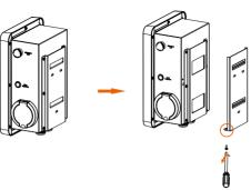
STEP 2: Fix the back bracket and the cable hook (only for Plug Type) to the wall.
