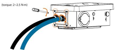
STEP 12: Hang the EV-Charger up carefully and steady the EV-Charger with the self tapping screw and the cross screwdriver.
