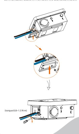
STEP 11: Push the rear cover to appropriate position of the cables and screw the self tapping screws with the cross screwdriver. Then tighten the waterproof fastening heads.
