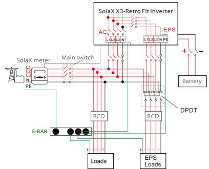
**Digram B** applies to the wiring rules which requires Neutral line of alternative supply must not be isolated or switched. (applies to wiring rules AS/NZS\_3000:2012 for Australia and New Zealand)
