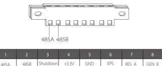
Note: 1 and 2 are the function interface of electricity meter; 3 and 4 are intelligent switch interfaces; 5 and 6 are parallel interface; 7 and 8 are reserved interfaces.
