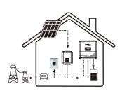
the power is not enough, battery will discharge for local loads first, and grid will supply power when power generated is not enough or battery capacity reaches too low.
