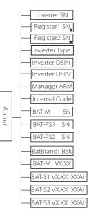
Register1 SN: it indicates the serial number of the external monitoring devices, such as pocket WiFi, pocket LAN and pocket GPRS.
