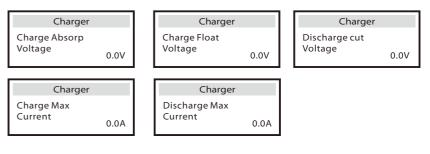
When the battery voltage reachs the value( discharge cut voltage for lead-acid battery, min capacity for lithium battery) in on-grid mode, battery will stop discharging and the system will go into IDLE mode.
