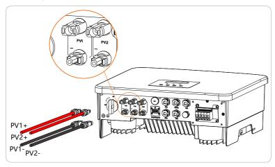
Schematic diagram of the inverter PV connected.
