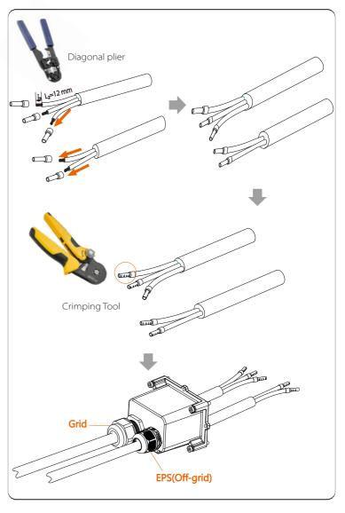
**Step 4.** Find the location of the AC interface on the inverter, insert the crimped terminals into the UW10 terminals L, N, and P according to the wire sequence, and use a flat-blade screwdriver to tighten the screws. (Torque: 1.5±0.1 N·m)
