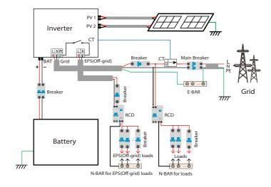
Diagram B: Neutral line and PE line are separated from each other, all loads connect to the EPS(Off-grid) port; (For most countries)
