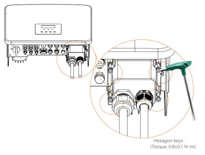
Step 6. Tighten the waterproof fastening head.
