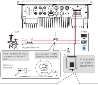
If the user has other power generation equipment (such as inverter) at home and wants to monitor both, this inverter provides CT2 communication function to monitor the power generation equipment.
