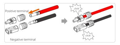
**Step 6.** Tighten the fastening head and insert into the corresponding positive and negative (PV+/PV-) ports of the inverter.
