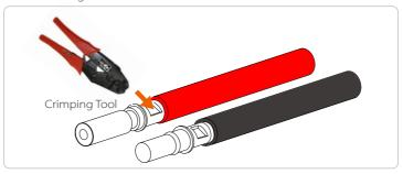
**Step 5.** The PV joint is divided into 2 parts - the plug and the fastening head. Insert the cable through the fastening head and the opposite plug. Notice that the red and black lines correspond to different of plugs. Finally, force the cable pair into the plug, will a "click" sound, which indicates that the connection is completed.
