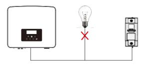
Figure: Wrong connection of load and inverter
