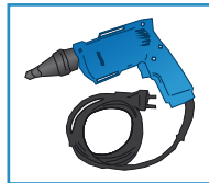
Power screw gun, preferably with depth stop
