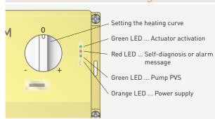
Self-diagnosis is performed when starting for the first time. The red LED flashes for about 5 seconds and goes out. After about 5 minutes the controller begins to adjust the flow temperature to the heating curve. If the red LED is continuously illuminated an alarm is present. In this case the wiring must be checked. An alarm occurs if the flow temperature in the surface heating circuits exceeds 55 °C. The controller returns to normal operation when the flow temperature cools to below 52 °C.
