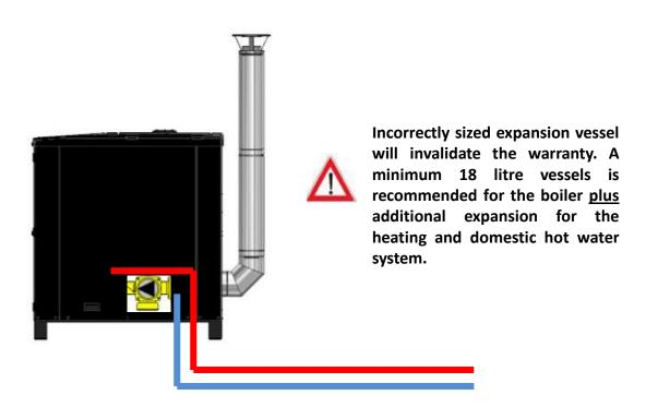
The boiler can be plumbed into either an open vented system (the maximum static head of water permissible is 90 ft. (27.44 meters) or a sealed system. If plumbed into a sealed system an appropriately sized expansion vessel should be used and installed as per manufacturers instructions. The expansion vessel should be sized based on the water capacity in the boiler and the water in the entire heating system.
