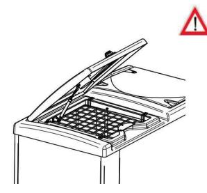
Never allow any foreign material to enter the hopper. This will lead to the malfunction of the auger system and could cause damage to the appliance and invalidate your warranty.
