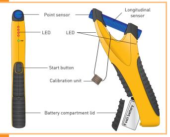
The Variotherm pipe locator detects VarioProFile pipes 16x2 / 11.6x1.5 and Variomodular pipes 11.6x1.5 in:
